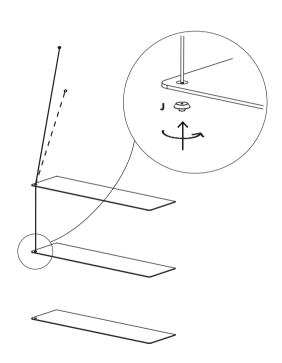
TAKE THE CONNECTOR WIRE THROUGH THE HOLE IN THE BOTTOM SHELF AND ATTACH THE BOTTOM METAL CONNECTOR CAP.
